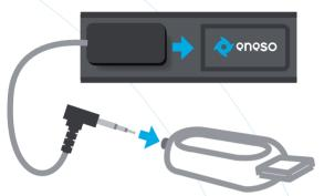
Insert the sensor into the band pocket and connect it to the USB device.
